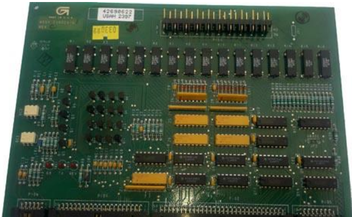
Gilbarco Highline / Dimension Assy dispenser board
