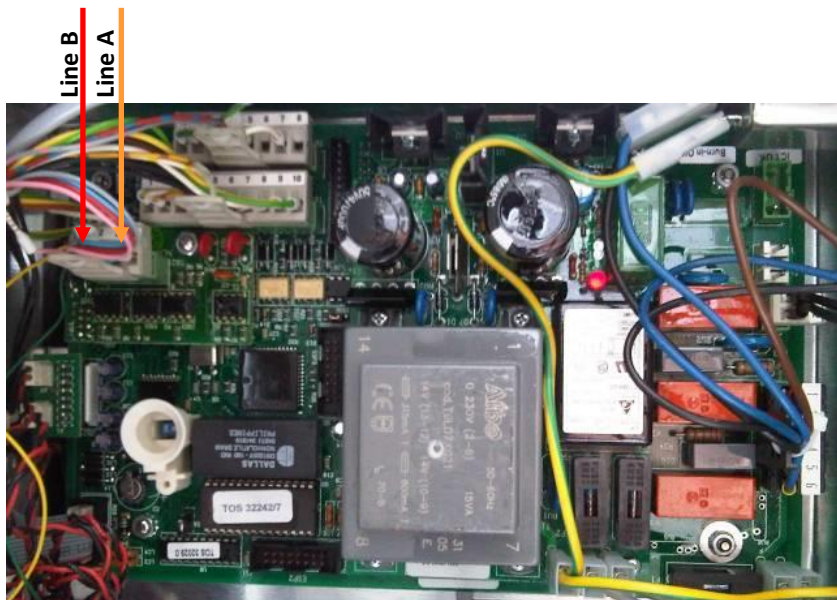
Nuovo Pignone monoprodukt dispenser board
