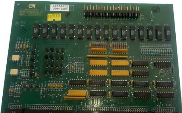
Gilbarco Highline / Dimension Assy dispenser board
