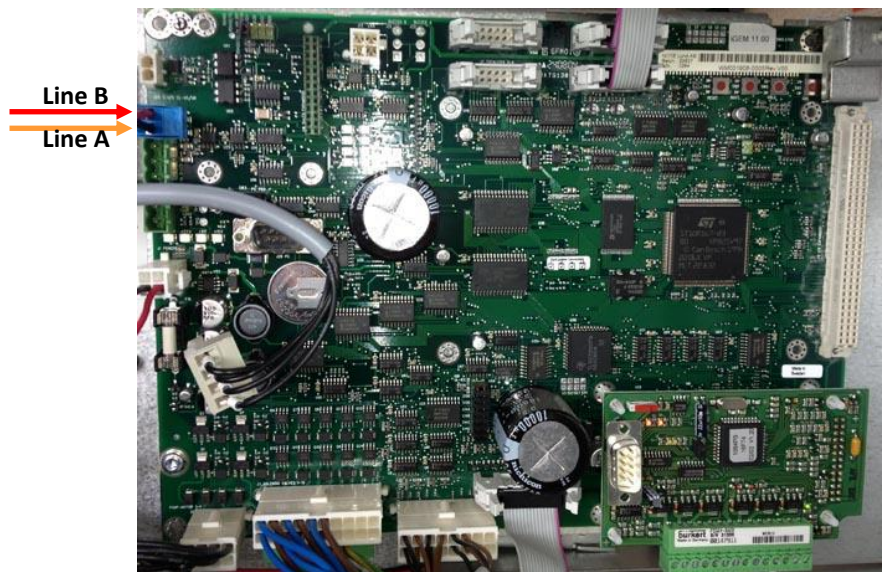
Mepsan dispenser board
