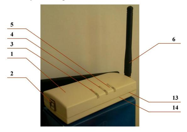
RF-hub is performed in a plastic case (1) of white color. Power supply is made through the USB-connector (2). Transfer and reception of data to RF-hub through a wireless interface is performed through HF-antenna (6) connected through SMA-jack (17). Means of indications are located on front surface of case — red LED "Status" (5), blue LED "Tx" (4) and green LED "Rx" (3). Holes for buttons "Reset" (13) and "Loading" (14) and located on side surface of case.
