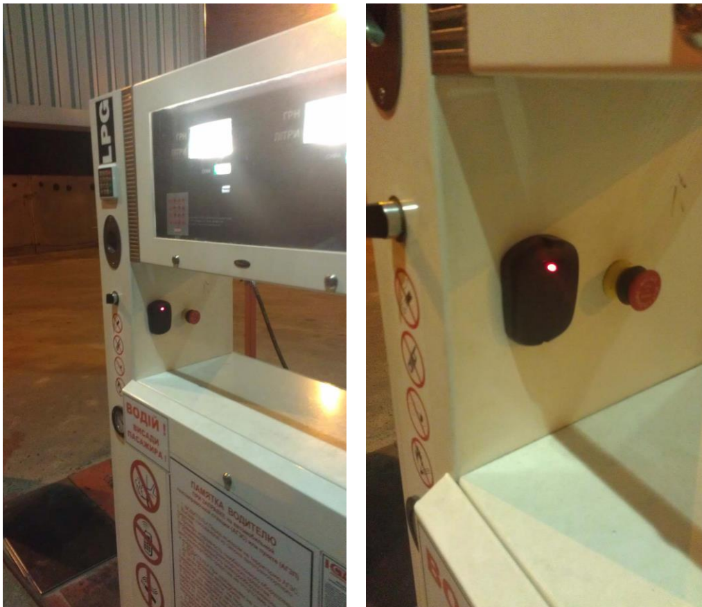
Example of reader installation on fuel dispensers
