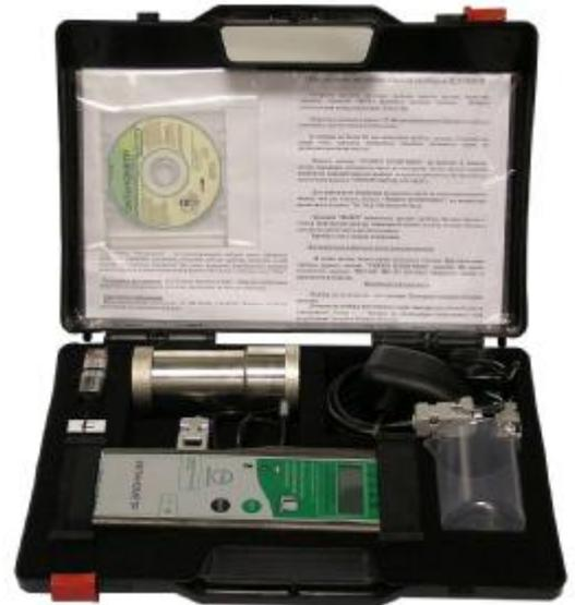
Software on a CD for work on the personal computer in Windows XP is supplied together with a octane number meter
